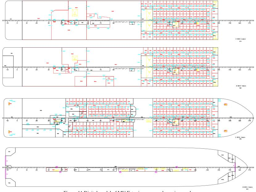
Figure 11 Digital model of MV Estonia, space and openings codes
