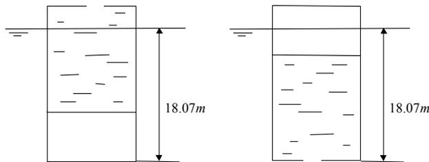
Figure 2: A barge with superstructure at upright floating and upside down attitudes
