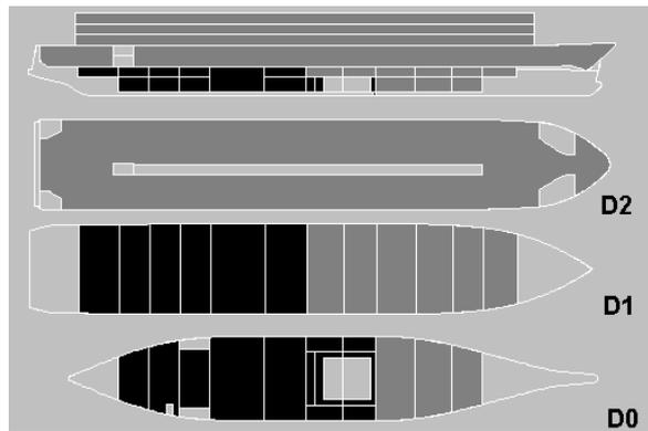
Figure 6: Aft spaces (AS) below CD flooded
