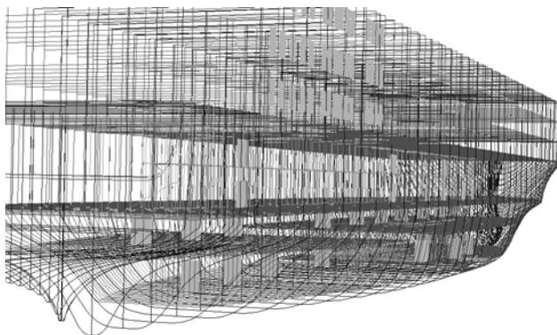
Figure 13: Numerical model of geometry of MV Estonia
