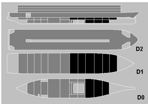
Figure 5: Forward spaces (FS) below CD flooded
