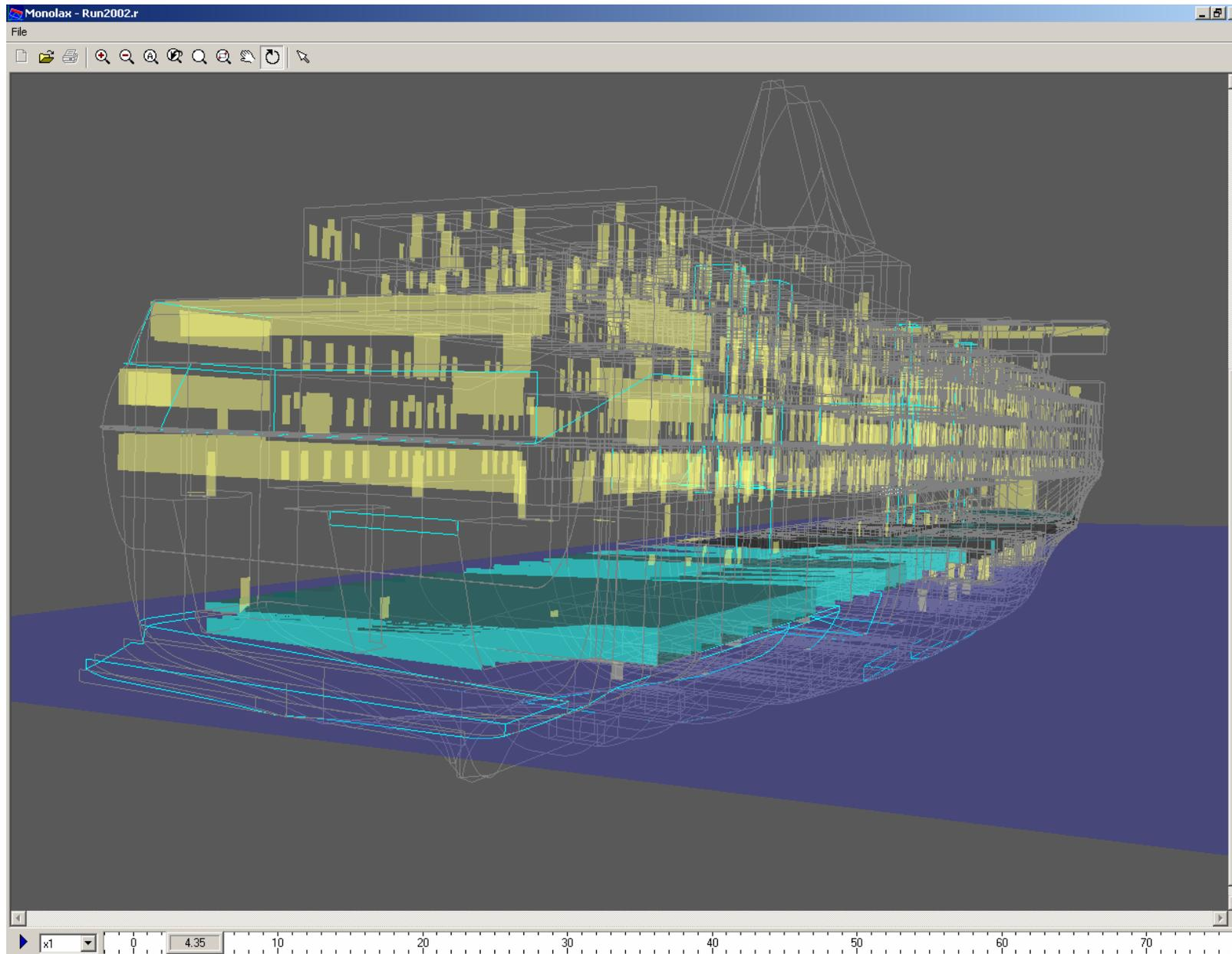
Figure 6 Flooding post-processing, virtual model of MV Estonia, aft view, MONOLAX, [www.safety-at-sea.co.uk](http://www.safety-at-sea.co.uk)
