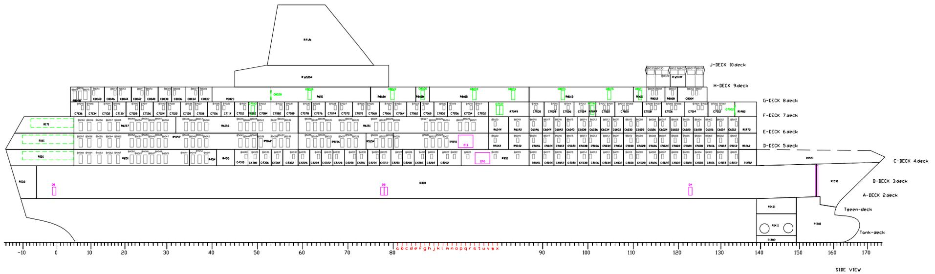
Figure 9 Digital model of MV Estonia, space and openings codes
