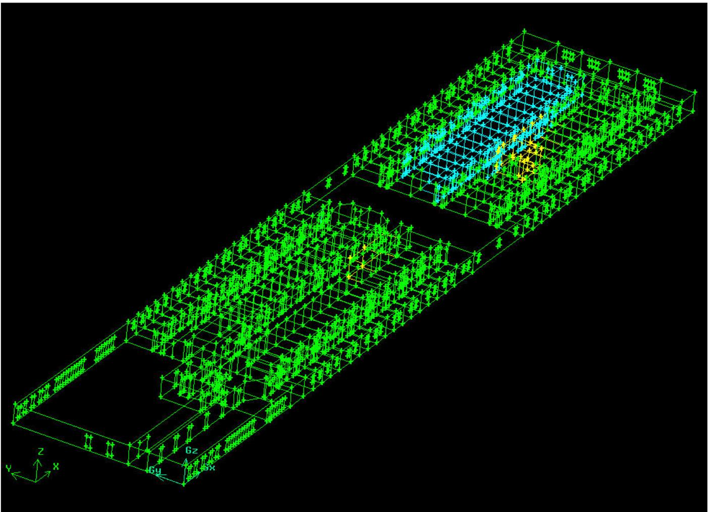
Figure 22 Deck 4 without all watertight sections and cabins, FLUENT model
