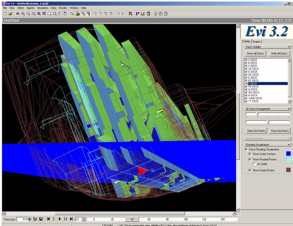
Figure 3 Combined flooding and evacuation models of MV Estonia - PROTEUS3 and Evi 3.2
