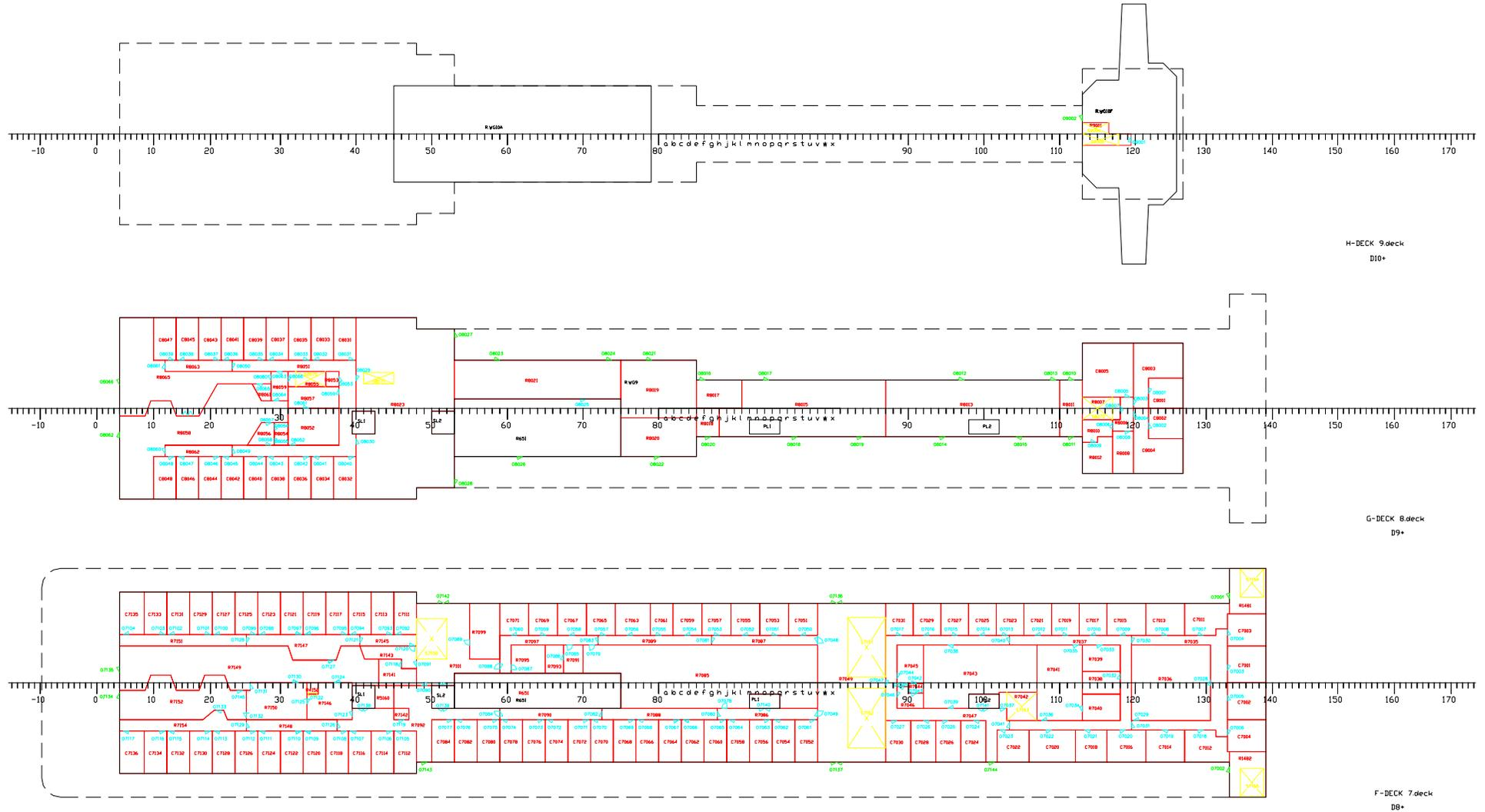
Figure 10 Digital model of MV Estonia, space and openings codes
