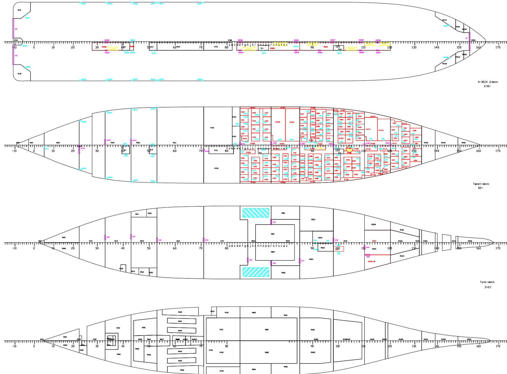
Figure 12 Digital model of MV Estonia, space and openings codes
