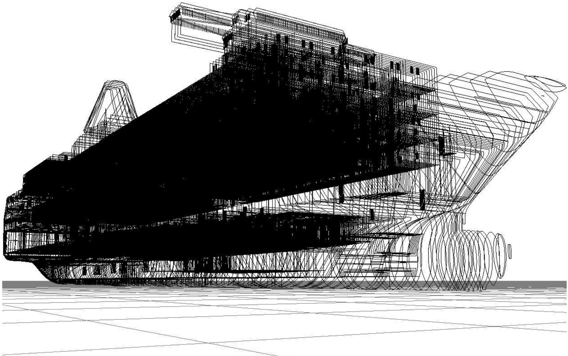
Figure 4 Digital model of MV Estonia, front view, PROTEUS3, [www.safety-at-sea.co.uk](http://www.safety-at-sea.co.uk)
