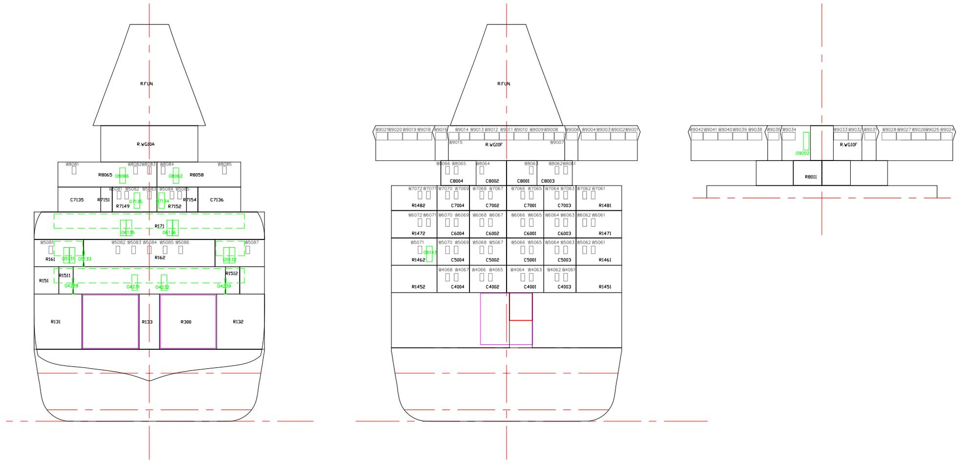
Figure 8 Digital model of MV Estonia, space and openings codes
