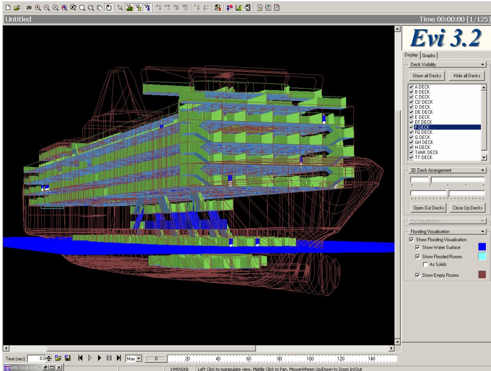
Figure 21 Combined evacuation and flooding model of MV Estonia, forward view, 126 survivors distributed as reported in [ 1 ], Evi 3.2 and PROTEUS3, [www.safety-at-sea.co.uk/evi](http://www.safety-at-sea.co.uk/evi)
