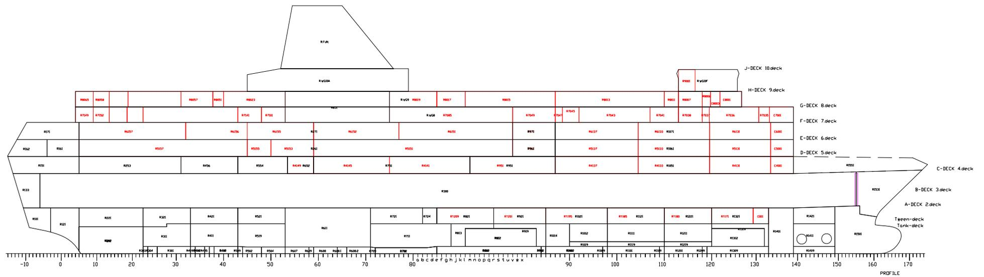
Figure 7 Digital model of MV Estonia, space and openings codes
