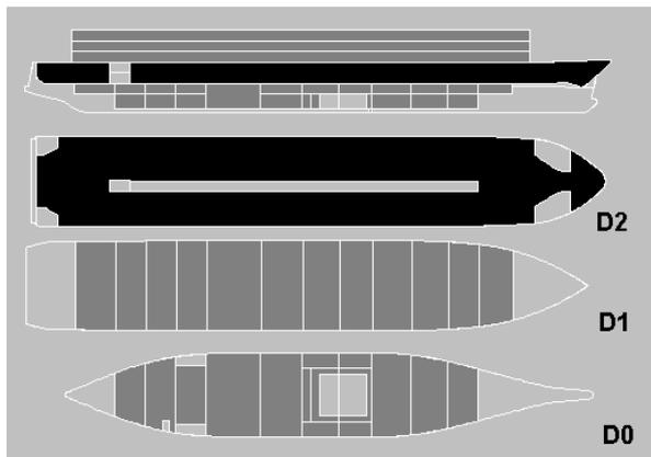
Figure 4: MV Estonia with Car Deck (CD) spaces flooded
