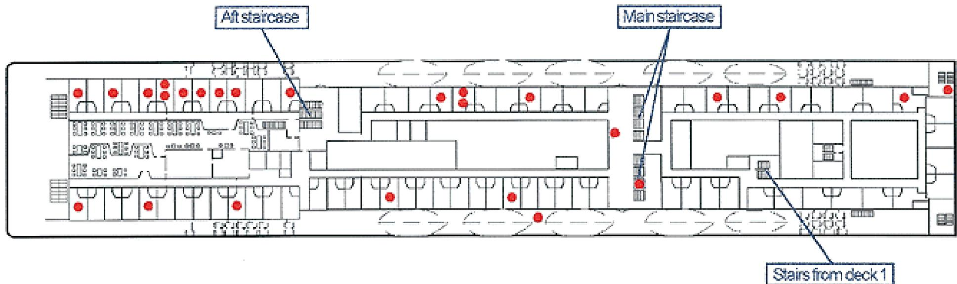
Figure 14 Plan showing deck 7, escape routes led to 18 rescue station located on this deck, red dots mark all known locations of **26** survivors at the onset of the accident, [ 1 ]
