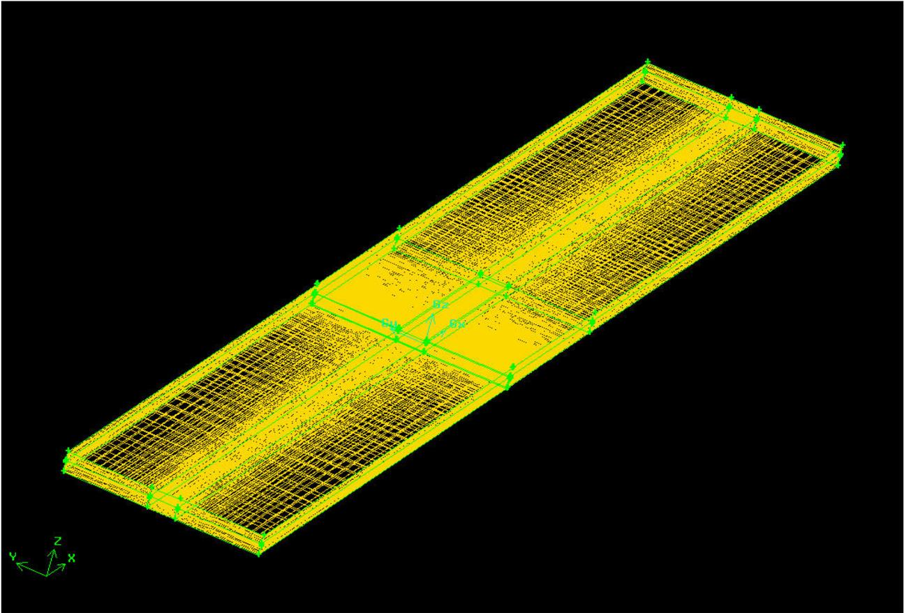
Figure 23 Deck 4 without all watertight sections and cabins in the water/air domain, FLUENT model
